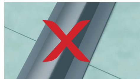
Do not install EJObar over the seam, without using an additional membrane cover strip.
