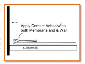
**INSTALLING A WALL TRIM** –After adhering the membrane up the vertical wall, trim the membrane and fit the Wall Trim into the preprepared groove in the mortar join or render. The Wall Trim can be secured using self-sealing hex screws at 1500mm intervals.
