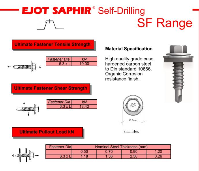
Figures taken from Steel designated as minimum yield strength 220Nmm<sup>-2</sup>
