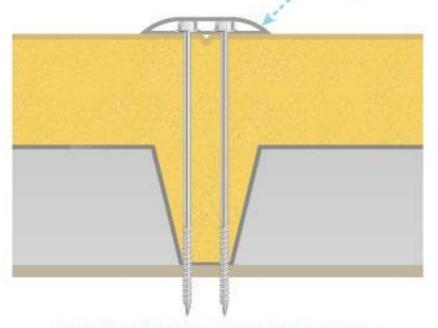
For faster installation, one X Plate washer positions the fasteners at 30mm centres to aid installation into a 40mm wide Profile.
