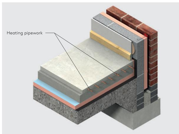
Figure 8: 24 Hour Heating Application - Below the Floor Slab
