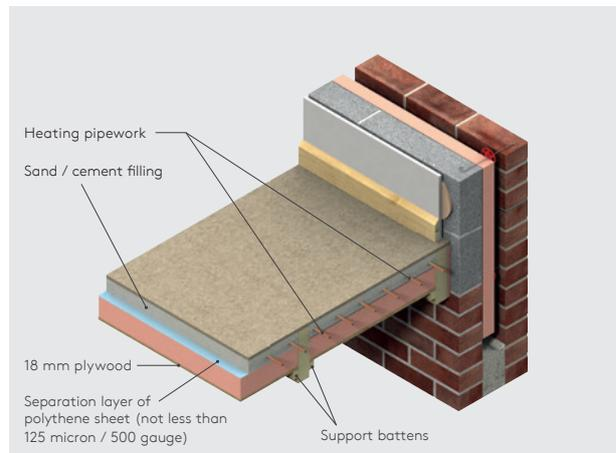
Figure 11: Intermittent Heating Applications - Suspended Timber Floor
