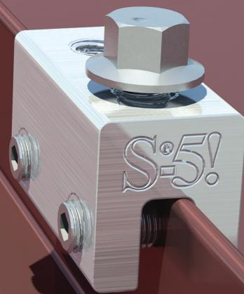
The S-5-E clamp is secured with our patented round-point setscrews without piercing the metal roof panel, thereby preserving the roof's warranties!
